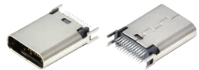
533 USB Type C Receptacle Vertical Height:10.5mm Positions:24
