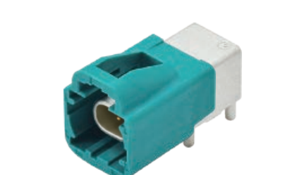
544 HMTD-N Plug 1x1 Right Angle Type Coding:A,B,C,D,E,F,G,H,I,J,K,L,M,O,Z Positions:02
