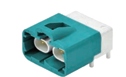
544 HMTD-N Plug 1x2 Right Angle Type Coding:A,B,C,D,E,F,G,H,I,J,K,L,M,O,Z Positions:04
