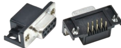
502 D-Sub PCB Right Angle Footprint:10.3mm(0.405") Positions:09,15,25,37
